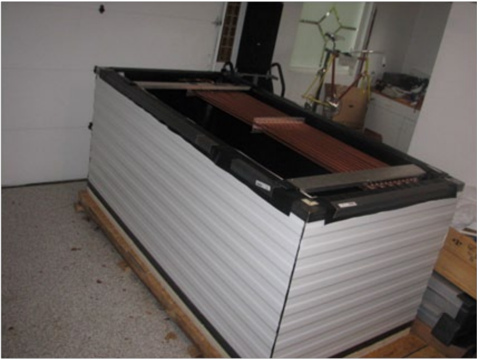
Figure S6: Prototype tank showing copper heat exchanger at top
