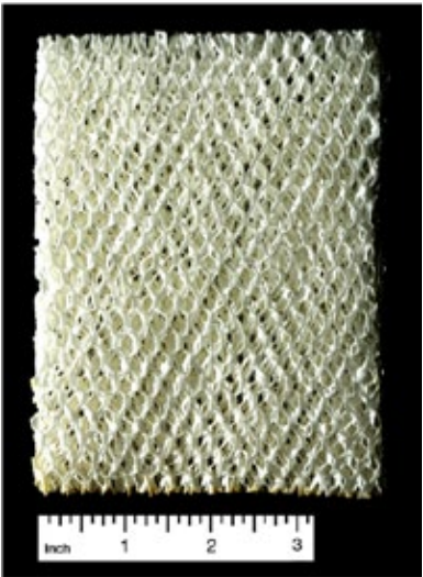
Figure L1: Sample of cellulose humidifier pad composed of hard and soft wood fibers.
