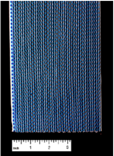
Figure L2: Sample of polypropylene humidifier pad.
