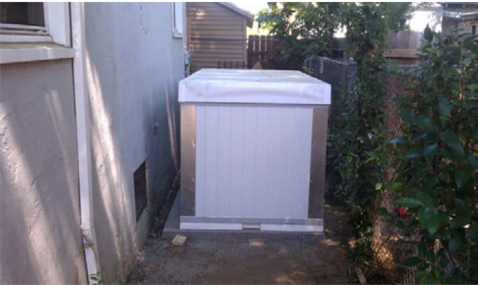
Figure S8: Tank in situ at field test site. The water in the tank is used to cool water pumped through the panels which are mounted on the ceiling, as the radiant cooling section.
