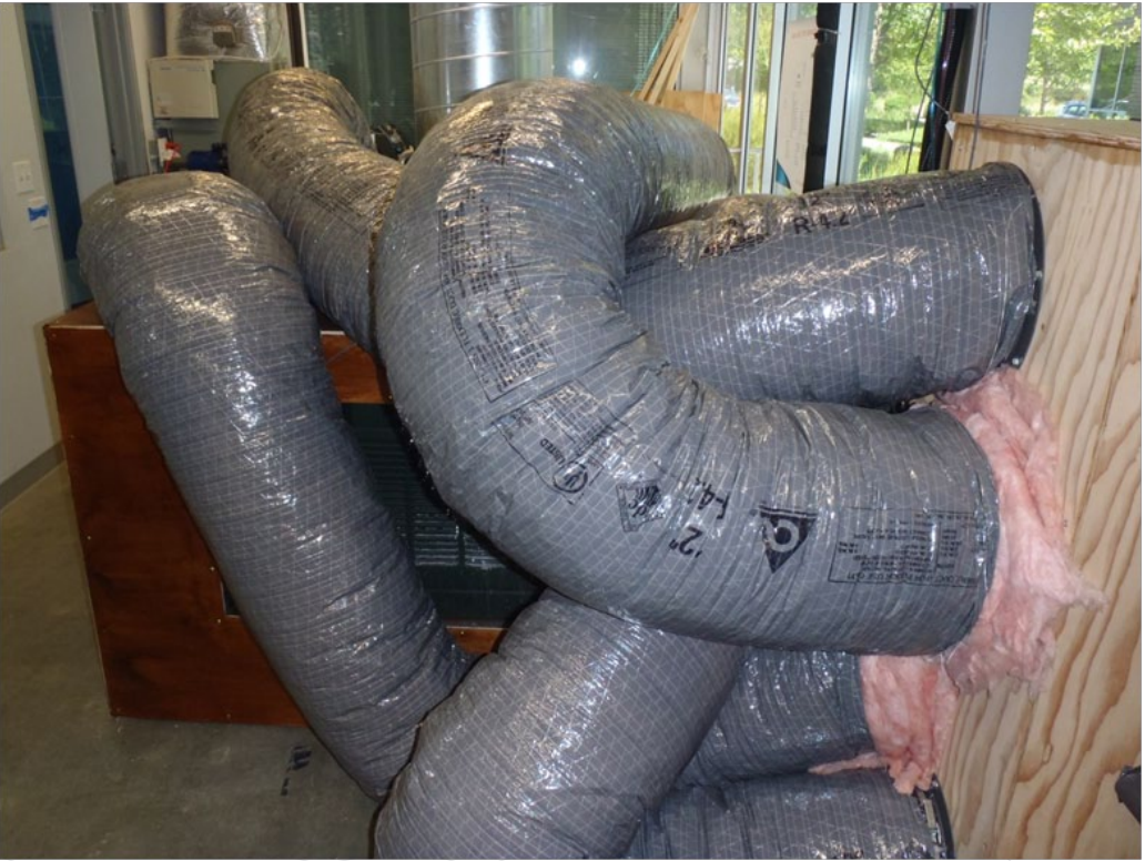
Figure S10: Aquachill in its temperature controlled box, with insulated ducts supplying temperature controlled air
