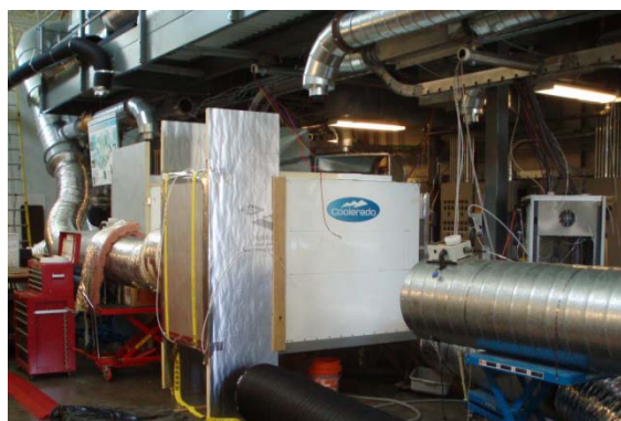
Figure 1. The prototype RTU and the unit being tested at the NREL HVAC laboratory
