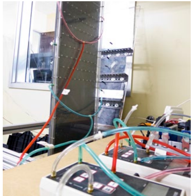
The test apparatus and sensors to determine pressure drop changes via pin distribution.
