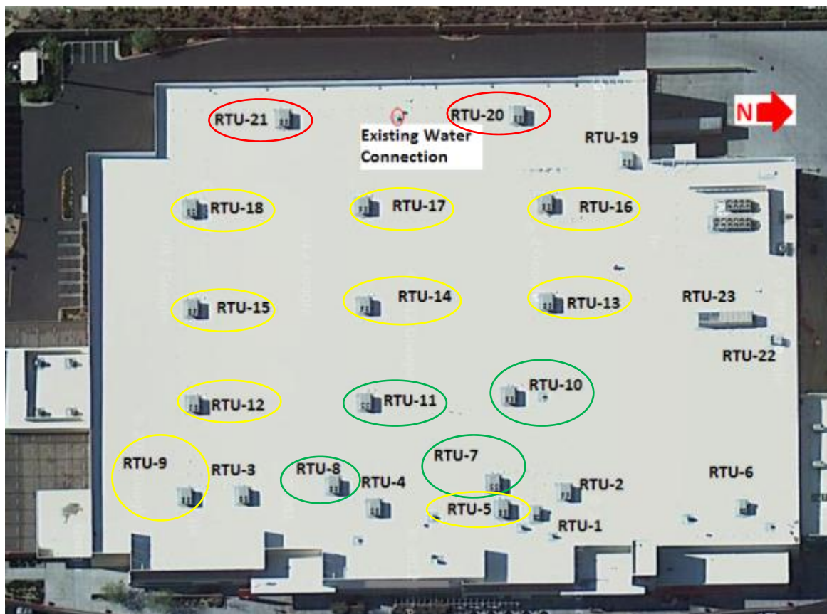
FIGURE 2: LAYOUT OF RTUs ON THE BIG-BOX BUILDING TESTED IN PALMDALE, CALIFORNIA. RED = BASELINE UNITS, GREEN = RETROFIT UNITS MONITORED, YELLOW = RETROFIT UNITS NOT MONITORED
