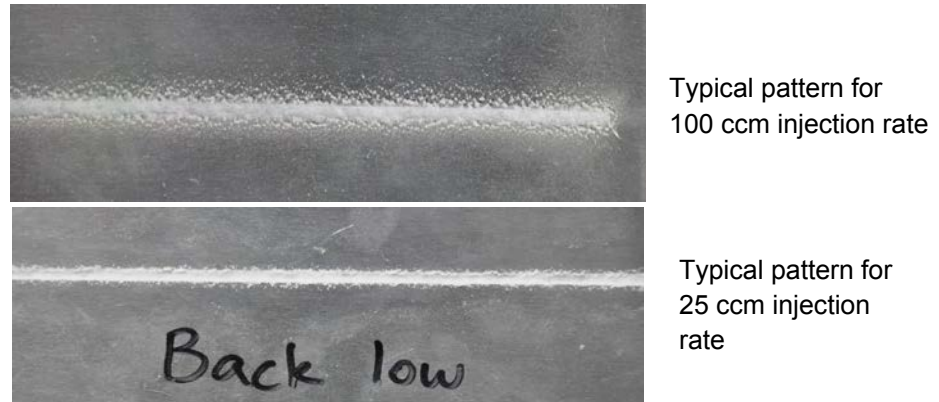
Figure 4. Sealant deposit pattern on back low panel for tests 1 and 2
