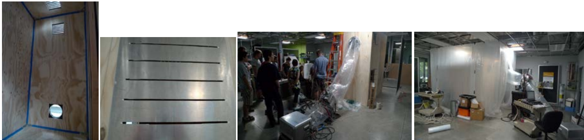
Figure 1. Photos showing the enclosure and leak panels used for the small-scale tests
