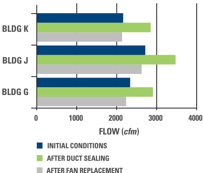
quality, and may result in less significant energy savings. For this demonstration fan flow was reduced by the volume offset by leak sealing, thus maintaining initial ventilation rates and achieving maximum energy savings.
