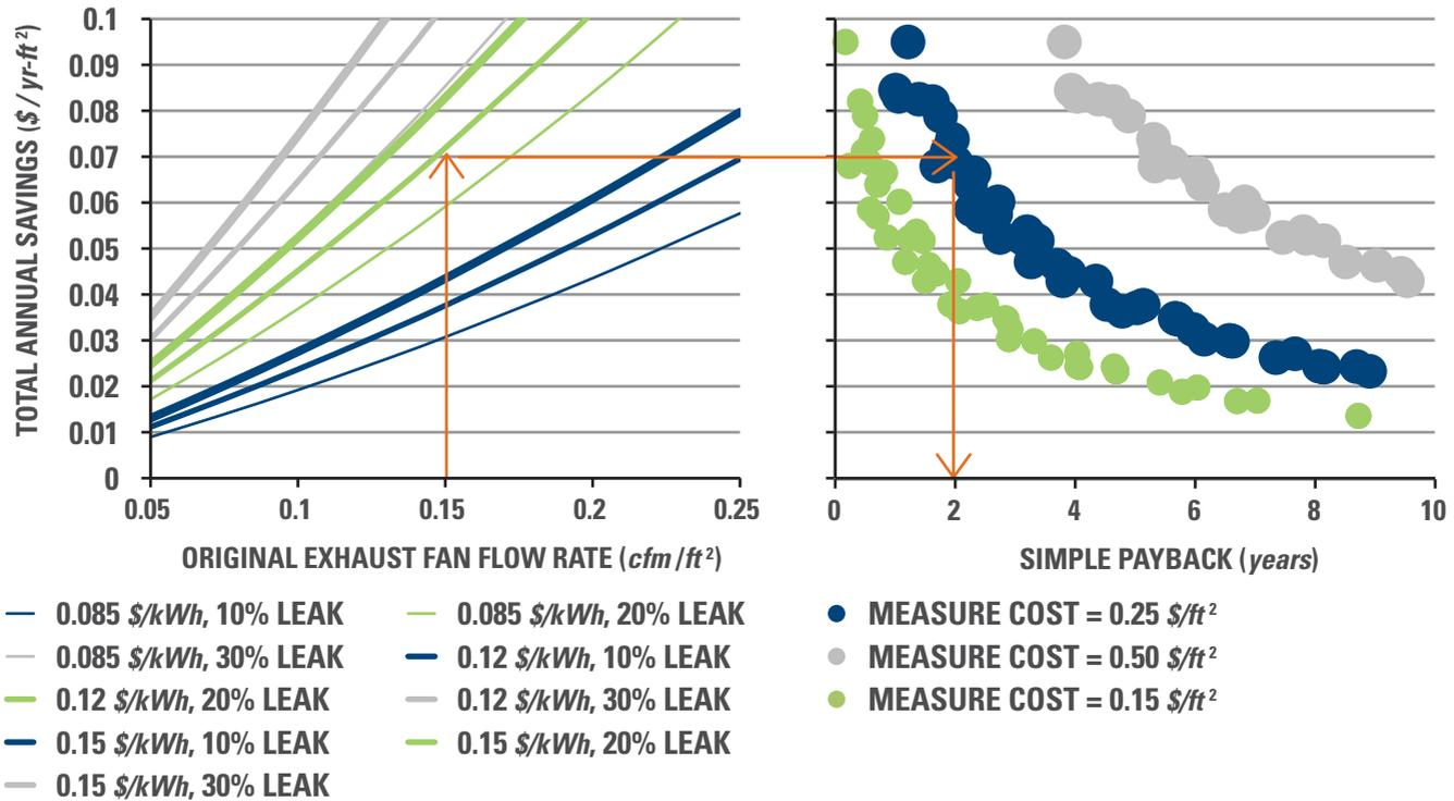
For the demonstration at UC Davis, estimated savings amount to more than \$3,000 per year. This amounts to a simple payback of 4.3 years or a debt service ratio of 43%. If the existing fans could operate efficiently at a reduced flow rate and replacement fans were not required, simple payback would be 2.3 years and the debt service ratio would be 23%.
