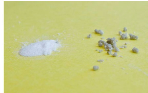
THE MPCMS IN POWDER FORM SHOWN BEFORE THE MECHANICAL CYCLING (LEFT) AND THE CLUMPS FOUND AFTER PUMPING (RIGHT)
