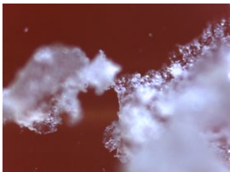
MICROSCOPE IMAGE OF WAXY CLUMP FOUND AFTER MECHANICAL CYCLING OF THE MPCM SLURRY
