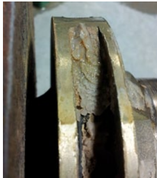
THE IMPELLER OF THE PUMP WITH WHAT SEEMS TO BE WAX FROM BROKEN MPCMS
