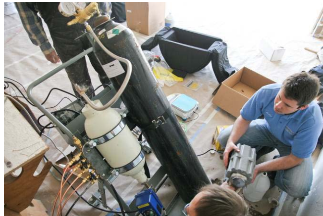
Figure 9. Multiple aerosol injection system developed by UC Davis.
