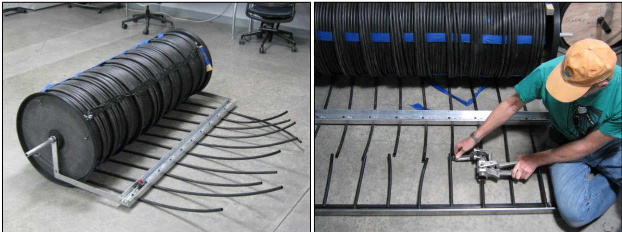
Figure 21 – Completed roll with 2.5 layers (left) and butt fusion of the manifold tubes to the spool (right).
