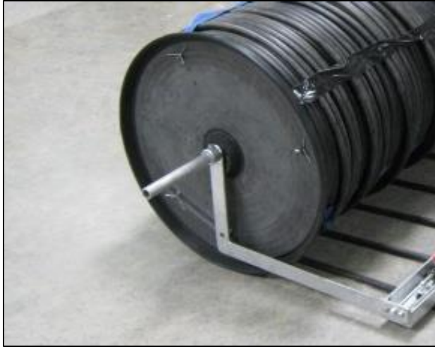
Figure 17 – Aluminum arms attach the rake to the axle with a location to attach the pull chain.
