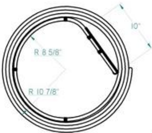
Figure 3 – End plate of 16 gauge steel sheet with clips to hold down return bends
