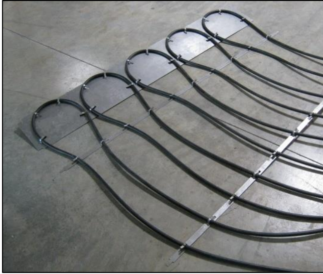
Figure 14 – Return bend stabilization consisting of end plate and two spacer bars with clips punched from sheet metal.
