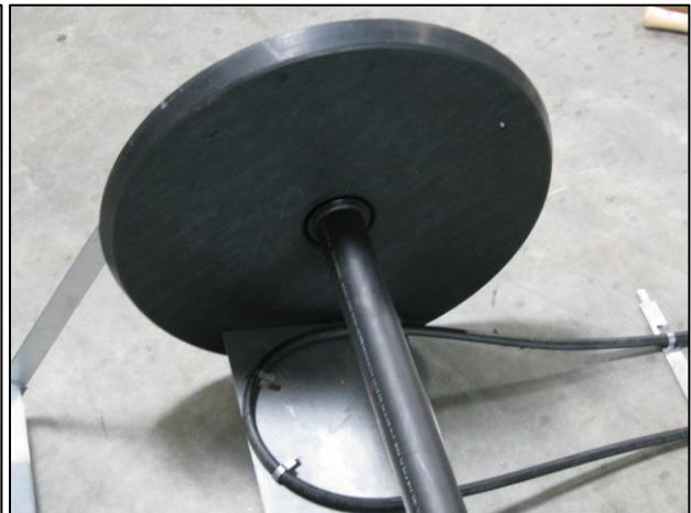
Figure 16 – Reusable rigid plastic wheel and axle sleeve assembly.
