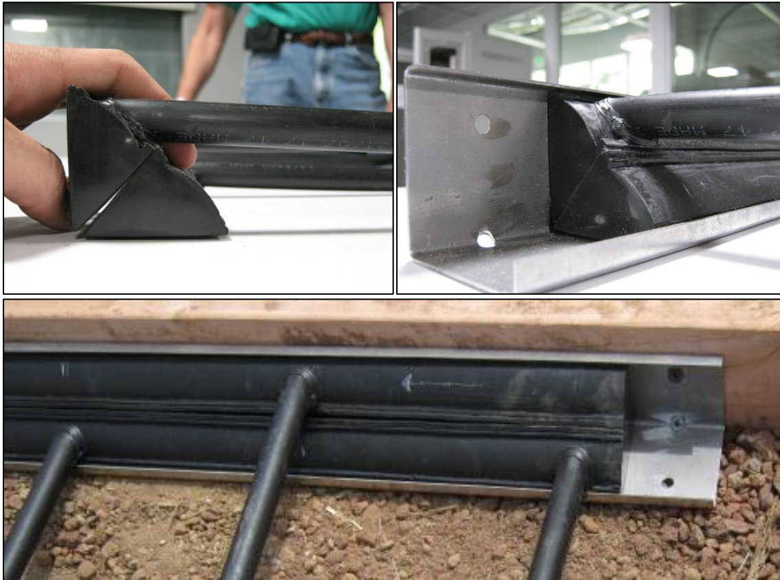
Figure 13 – Prototype of 5' manifold section with connections to tubing circuit.
