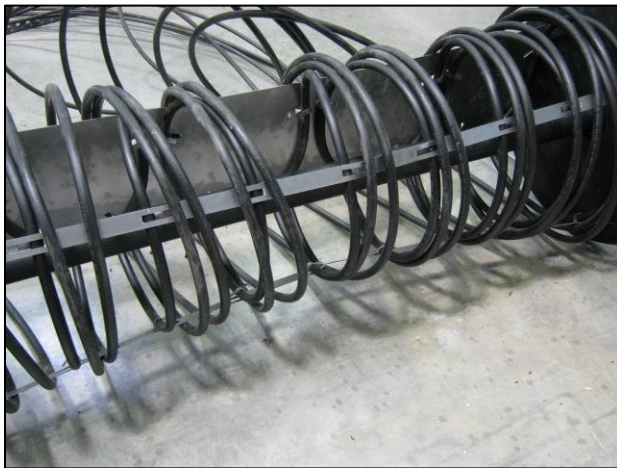
Figure 19 – Spacer bars and end plate deformed as the spool was rolled (left), so 2"x4"s were placed under the plates for additional support.
