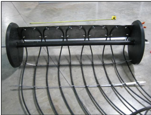
Figure 18 – Spool is assembled with end plate and two spacer bars inserted into the two wheels and pinned with cotter pins.
