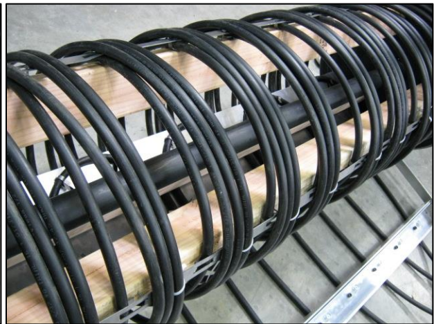
Figure 19 – Spacer bars and end plate deformed as the spool was rolled (left), so 2"x4"s were placed under the plates for additional support.
