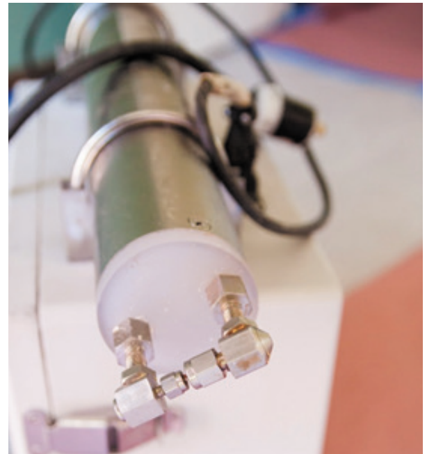
Figure 2: Close up of the sealant injector nozzle
