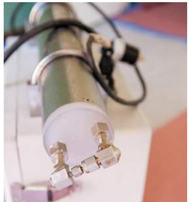
Figure 2: Close up of the sealant injector nozzle
