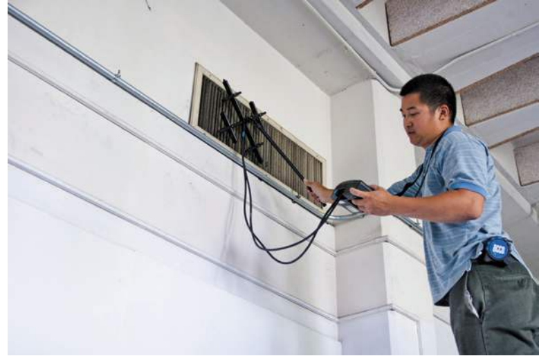
Figure 3: Pre-install testing and recording of flow rates from each of the registers in the building
