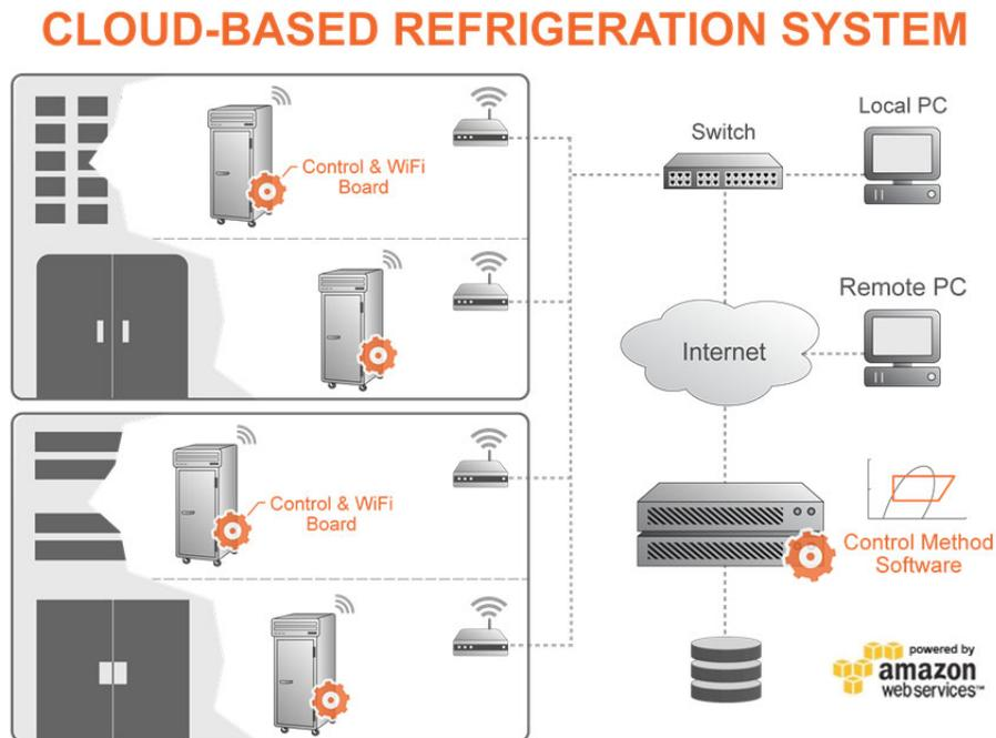
Figure 1. CloudFridge system diagram.
