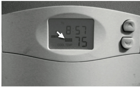
Fig. 2. Thermostat in hold mode (arrow) in a household reporting the use of programming features.
