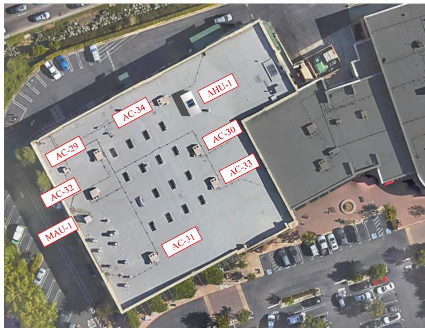
FIGURE 2. HVAC EQUIPMENT LAYOUT (GOOGLE 2015)
