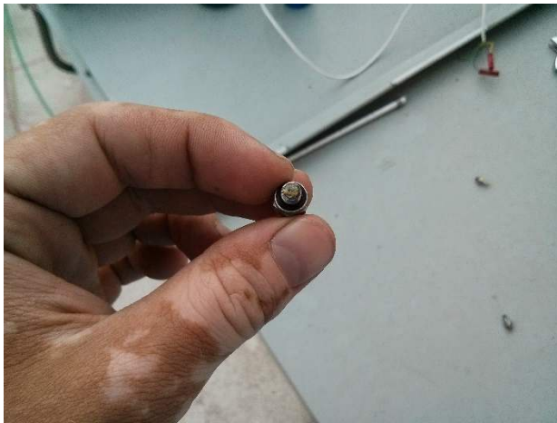
Figure 5: IEC water distribution system with clogged and cleaned adaptors
