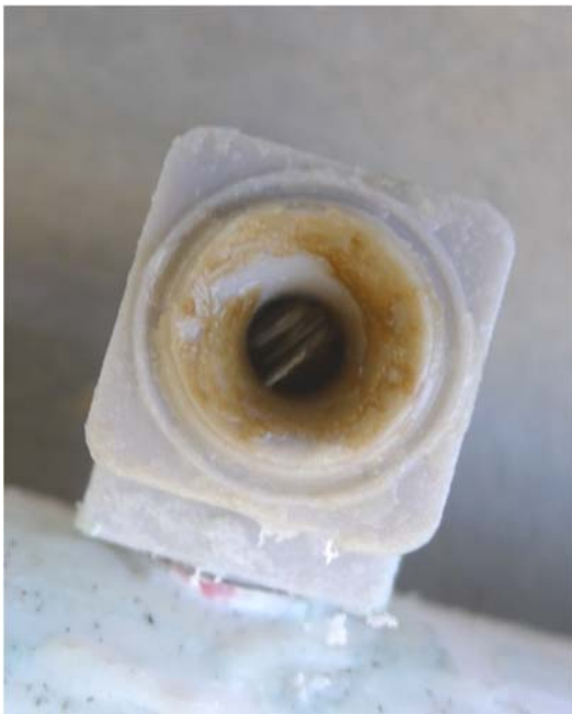
FIGURE 27. ECCU WITH LOW BLEED NOZZLE CLOGGING.
