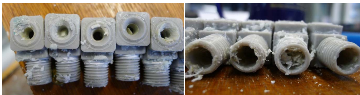
FIGURE 19. ECCU WITH NO BLEED NOZZLE CLOGGING.
