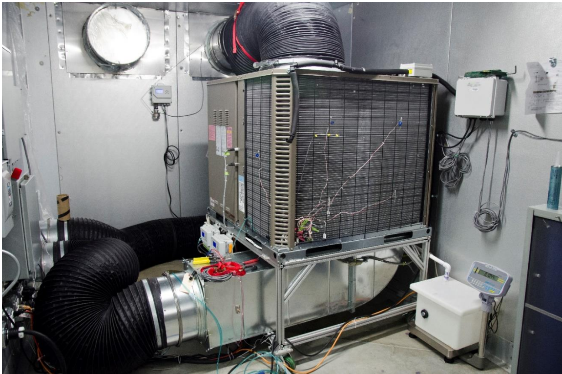
FIGURE 6: TEST UNIT INSTALLED IN THE ENVIRONMENTAL CHAMBER
