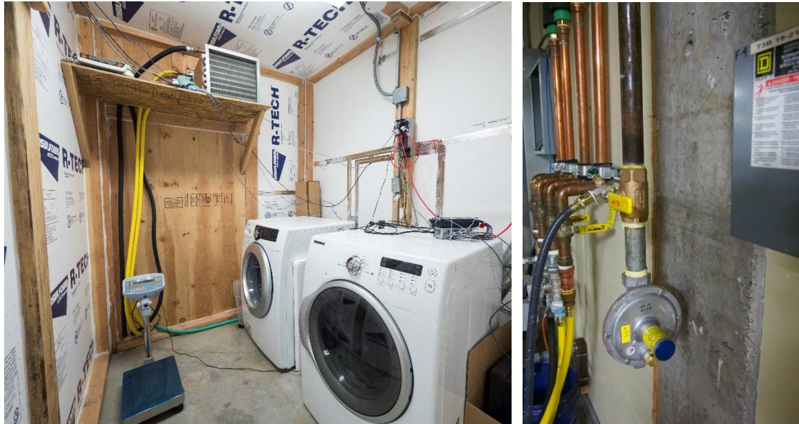
Figure 3 – Insulated wood frame chamber with heating, cooling, and dehumidification capabilities (left) and gas line and regulator (right).
