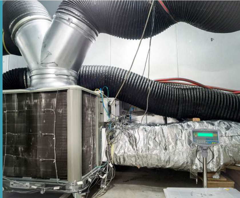
DR-55 refrigerant testing on a Trane heat pump in WCEC's environment chamber
