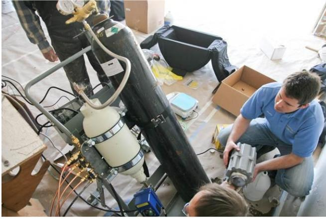
Figure 7: System developed by UC Davis, capable of multiple aerosol injection points
