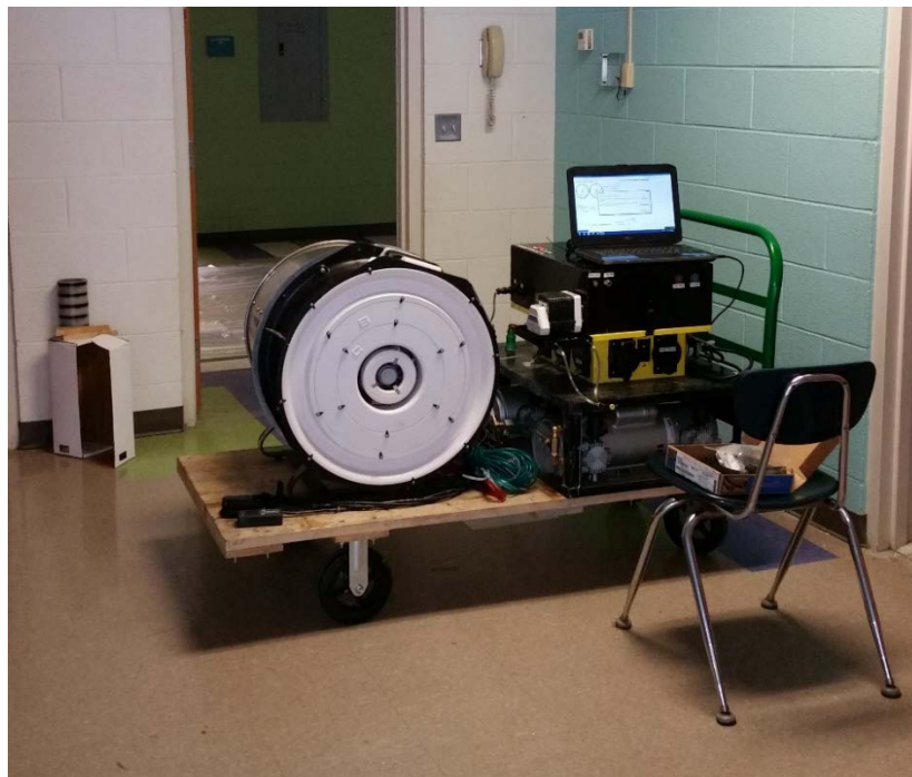
Figure 14: Photo of aerosol sealing equipment setup
