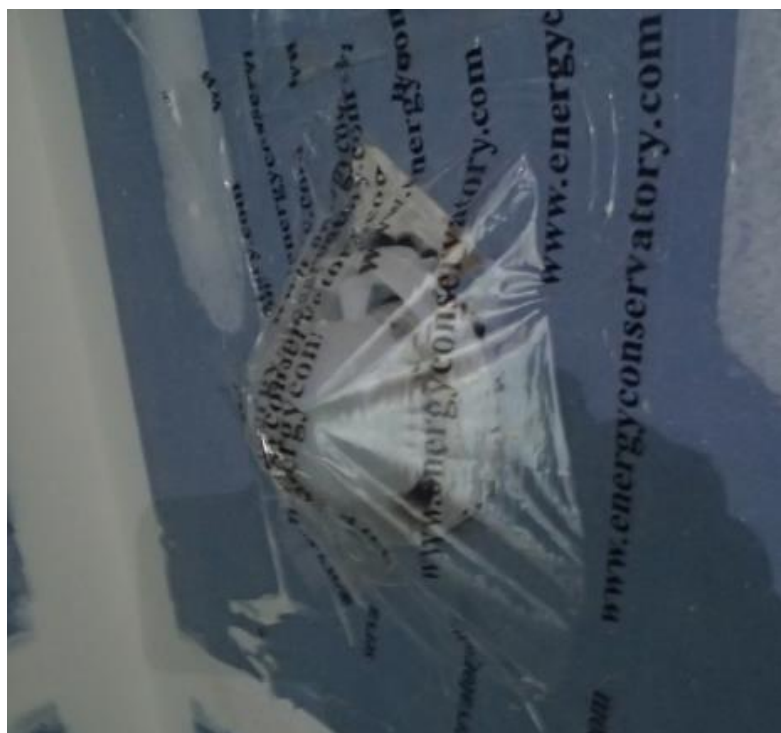
Figure 58: Shower handle temporarily sealed to protect moving parts and intentional leaks from being sealed
