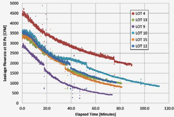
This plot shows the sealing profiles for each of the six aerosol envelope sealing demonstrations. The homes ranged from 2,000 to 3,500 ft<sup>2</sup> and were sealed after the drywall was installed and taped. Each home was sealed to 60%–85% of the initial leakage level in less than 2 hours; the average sealing rate was 290 cubic feet per minute (CFM) at 50 Pascal (Pa) every 10 minutes.
