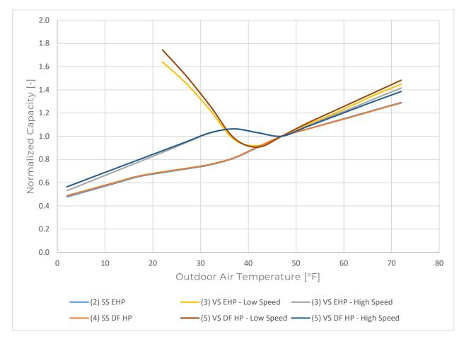
Figure 15 – Heat pump normalized heating capacity
