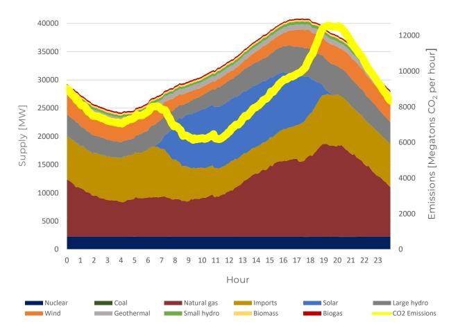
Figure 4 - Electricity generation and associated CO<sub>2</sub> emissions in California on August 10, 2018
